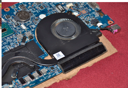
DESKTOP COMPUTERS (ABOVE) OFTEN HAVE LARGE HEAT SINKS WITH FINS ON THE CPU AND A FAN ABOVE THE HEAT SINK.
